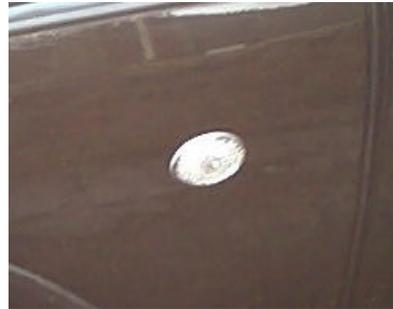
When the wiring is connected, switch on the hazard warning lights to see if the side repeaters work correctly.
